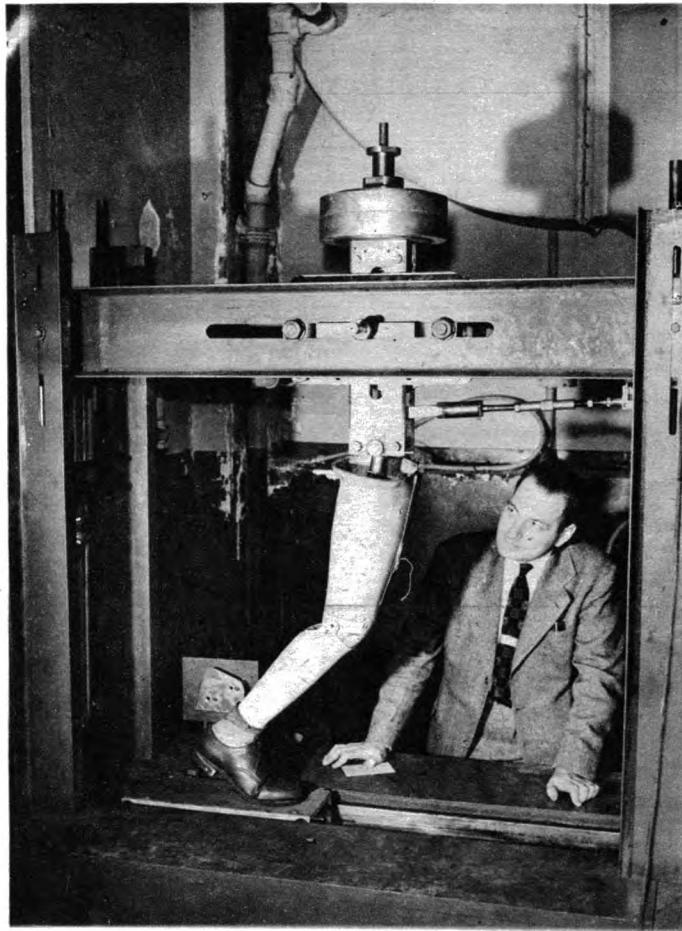
Artificial "testing" leg has taken 111,000 "steps" to determine construction and material weaknesses.
